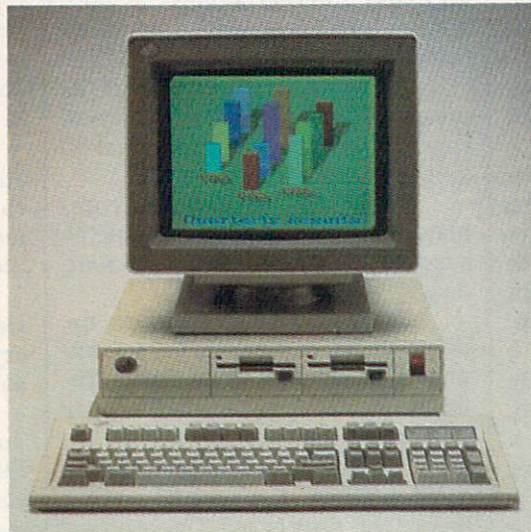
IBM's new System/2 computers are seen by some as an attempt to seal off the high-end business market, and by others as an invitation to create the next generation of clones and compatibles. The new Model 30 offers 640K RAM, color graphics, and three slots.
