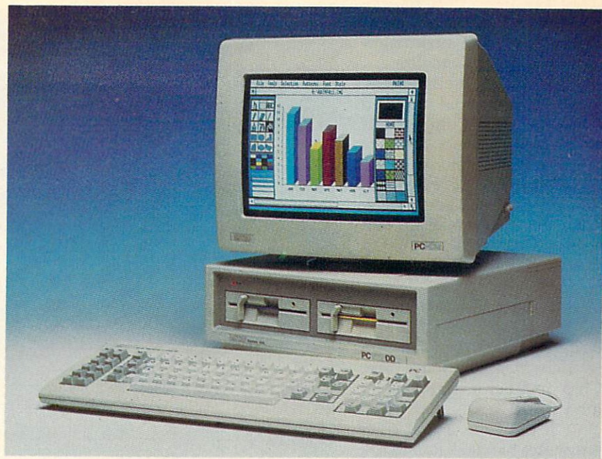
Amstrad has already sold many PCs in Europe. Its 1512 series offers a small footprint, and two operating systems, including Digital Research's GEM.
