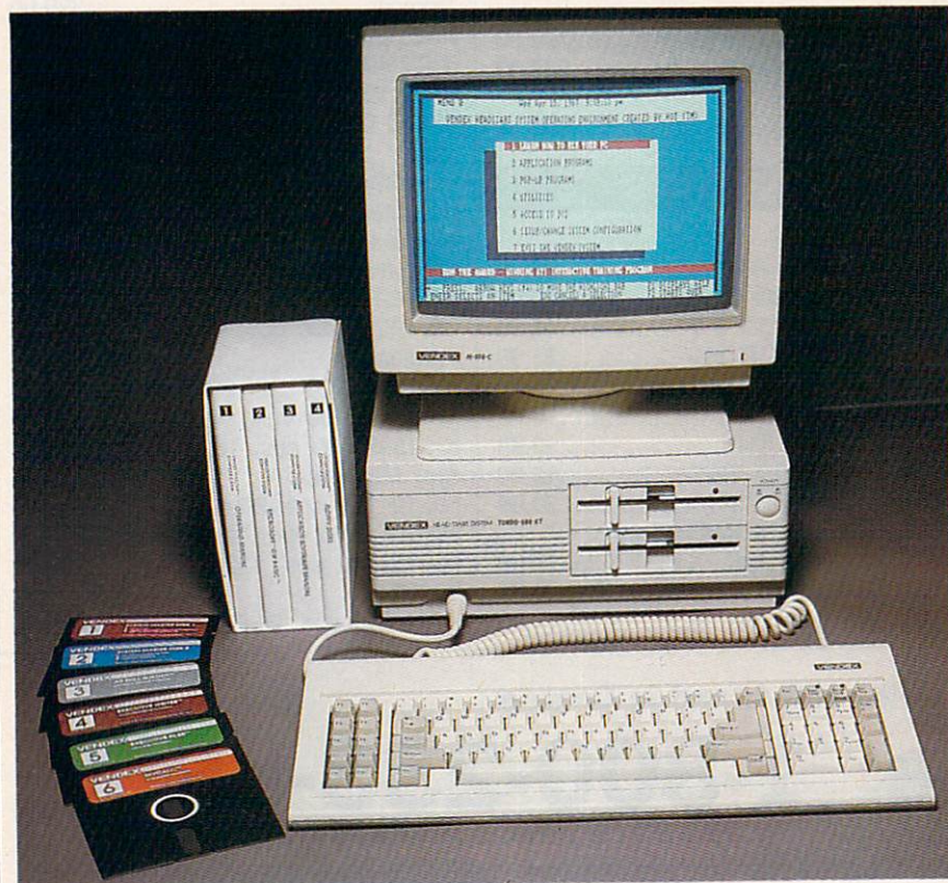
Vendex's computers, manufactured by Samsung of Korea, come complete with an on-screen manual, aimed at teaching the user while the computer is in use. The Turbo-888-XT features a full-size AT keyboard, 512K RAM, two 360K floppy disk drives, and MS-DOS 3.2.
