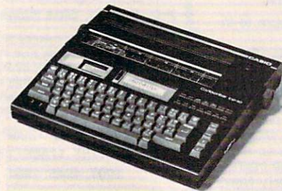
This Casio computer-compatible electronic typewriter is a hybrid—part typewriter and part word processor—that can connect to a computer to serve as a printer.
