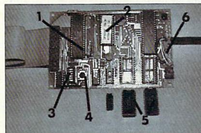
1 65C02 microprocessor; 2 8K interface ROM operating system; 3 setup switches; 4 reset pushbutton; 5 4K RAM buffer integrated circuits; 6 jack for power cable to cassette or joystick port.
