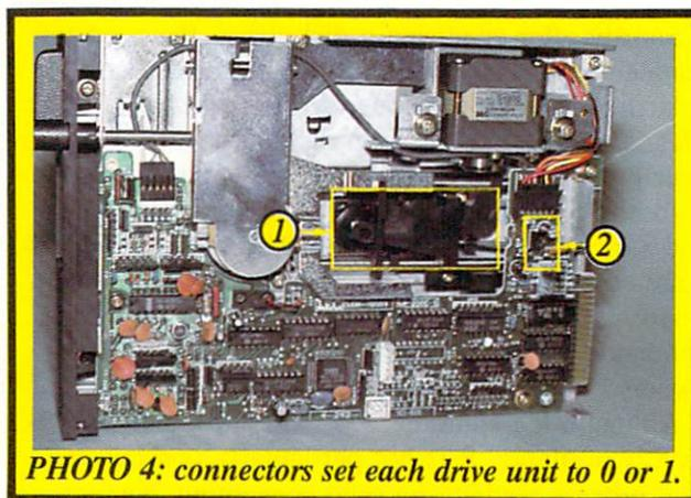
**PHOTO 4:** connectors set each drive unit to 0 or 1.
