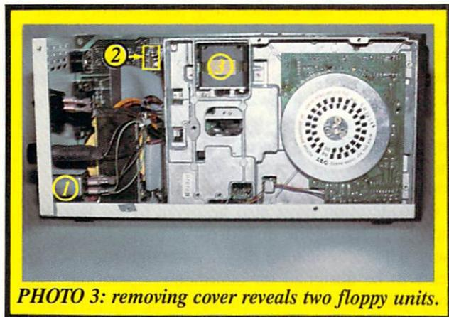
**PHOTO 3:** removing cover reveals two floppy units.
