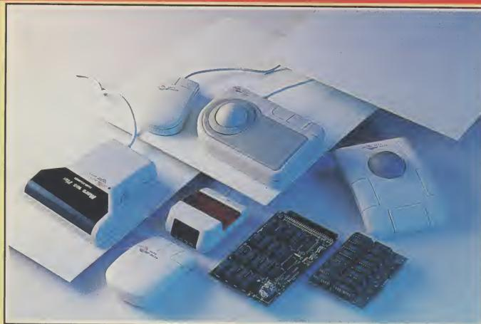
control with 280 dpi resolution, and doesn't consume much power by using the CMOS chip. A great little squeecker to have beside your machine. And the good news for Amiga and ST owners is that their version of the mouse is switchable between the two machines, and comes with a holder to keep it safe. PC owners get a dedicated mouse of their very own.
