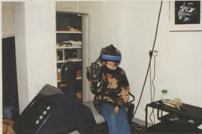
Bring on the Virtuality Force Feedback Glove. The version I tried was a little primitive but in was in the early stages of development. By using little airbags which inflate on command from the main unit the glove simulates contact with a solid object. It does not feel like the object touched (that is to come with a technique known as texture mapping which allows different surface areas of a solid to have their
