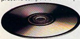
On a digital record, sound is carried by pits and spaces, which are read by a laser beam.
