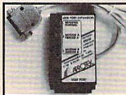
**NEW! "COM-MODEM" ADAPTER** — Use any Hayes® compatible modem with DB-25 connector through your USER port. You can make it emulate a 1670 too, or turn it off entirely. Can be used with our other USER port equipment such as "USER EXTENDER" (#5250) or "UNIVERSAL RS-232 INTERFACE" (#5232).
