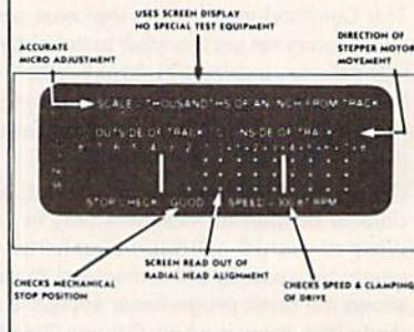
Package includes: • True digital alignment disk with offset tracks. • Mechanical Stop Test • Speed Test • Illustrated manual with instructions for performing alignment, adjusting speed and stop position. • Print test results for future reference.
