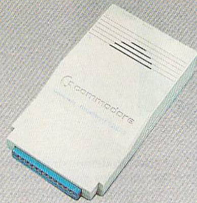
The 1670 modem from Commodore features 300/1200 baud, built-in speaker, auto answer, autodial, auto baud, and auto mode selection.
