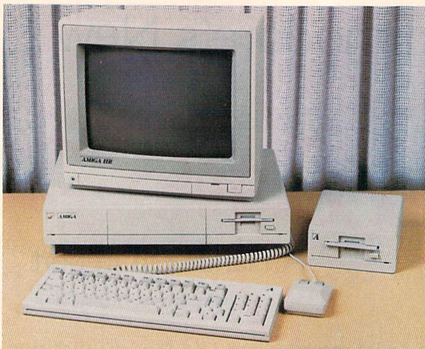
The Amiga computer from Commodore, with built-in 3 1/2-inch disk drive, detached keyboard, two-button mouse, and optional RGB monitor, and external drive.
