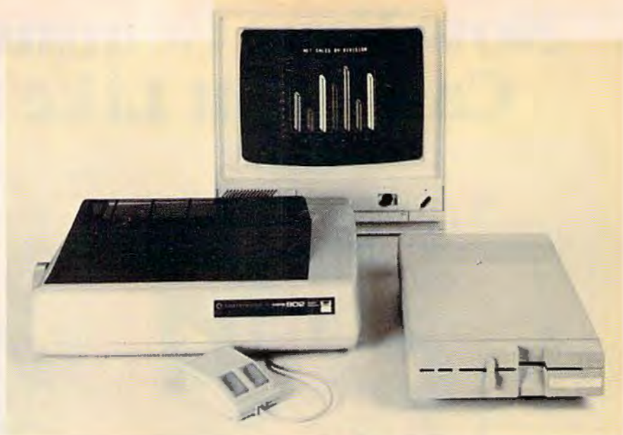
Among the new Commodore peripherals are the Mouse, MPS 802 Printer, 1902 RGBI/Composite Monitor, and the 1571 Disk Drive.
