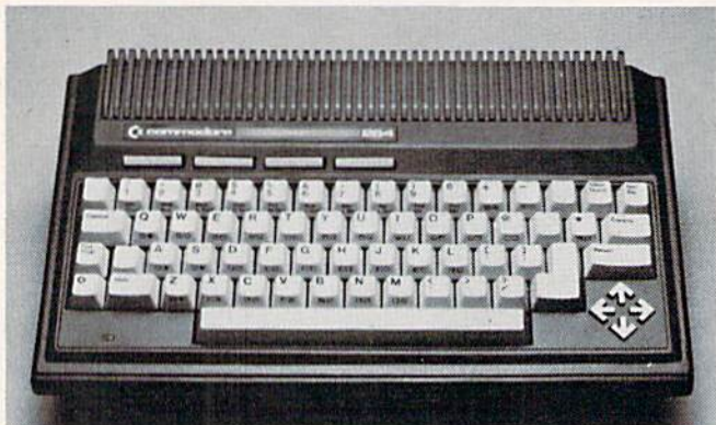
Commodore's new 264 computer, showing the four separate cursor keys (lower right) and the four programmable function keys (at left above keyboard). The Commodore 364 will have a similar console, but with a 19-key numeric keypad above the cursor keys.
