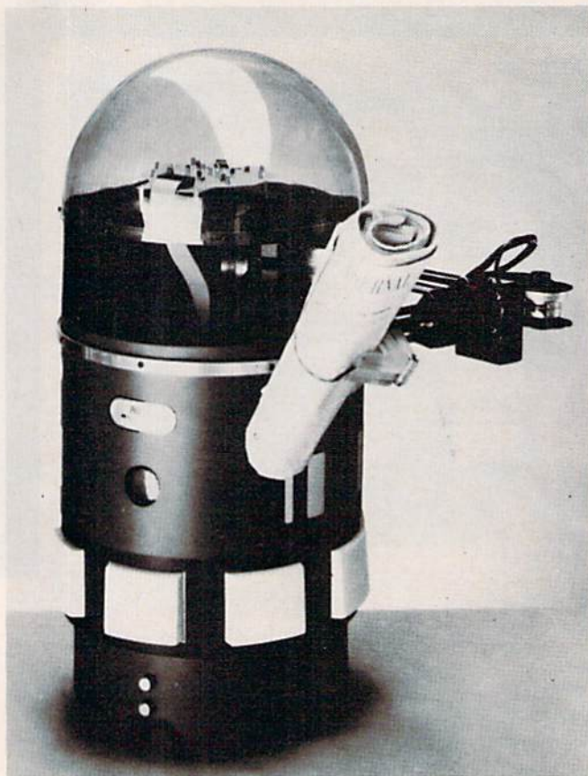
The RB5X, produced by RB Robot corporation, is a 23-inch-tall programmable robot, which can be plugged into a computer for instructions. Preprogrammed EPROM cartridges can also be used to direct the RB5X.
