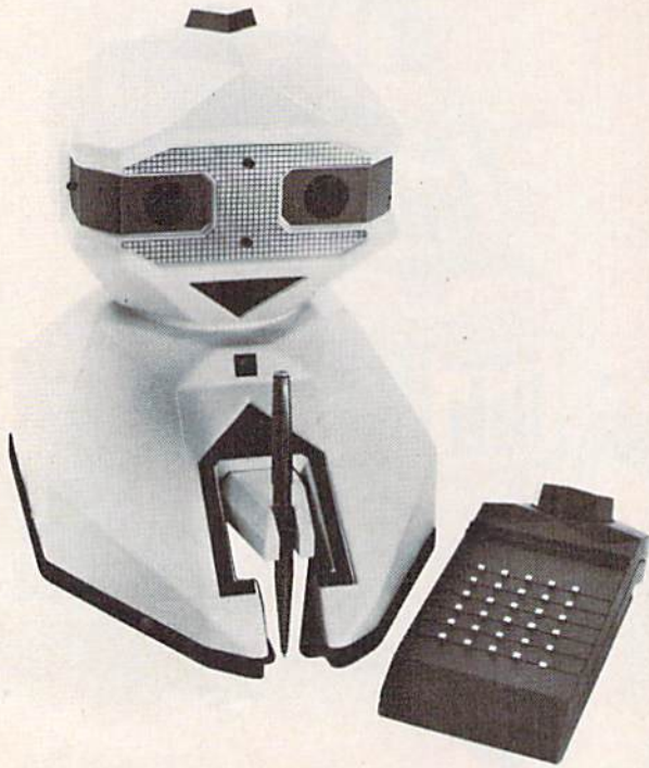
F.R.E.D. (Friendly Robotic Educational Device), a 12-inch, $349 robot that speaks, moves, and draws, and can be directed by an infrared signal from the remote control device at right.
