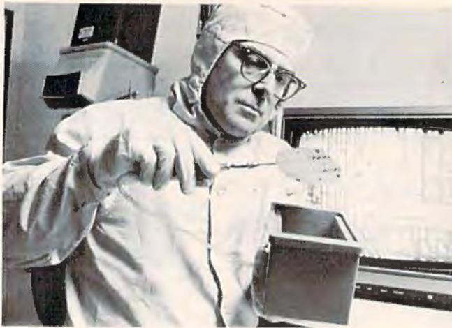
Engineer Mike Grieco at Bell Labs holds a wafer with 64 tiny chips. Behind him you can see a TV picture of the transistors on just one chip magnified 400 times.
