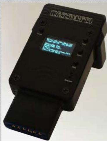
The wifi functionality can be used to upload a file onto your SD-card, but also to load a program via virtual file mode. Which is mostly interesting for people who like to program and want to try out their new software without loading it to the SD-card over and over again on every iteration of the code. Also thanks to the use of software exclusively written for the Cassiopei v2.0, you can use your it to play some fancy PETSCII video files (video only, no sound).
