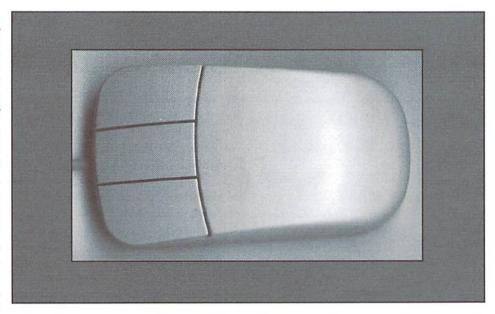
mouse over and remove the ball. The ball allows your mouse to "feel" how far it has moved across your mouse pad so it can tell the computer how far to move your pointer/sprite. The ball is usually held inside the mouse by a small plate that rotates or slides to a position where the ball can be removed by turning the mouse right side up. Don't forget to catch it, as losing the ball is the easiest way to ruin a mouse!
