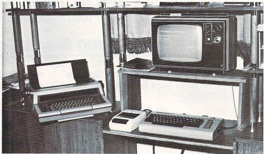
The SCM Typetronic fits in well with my C-64, Datasette and TV monitor. The Cord interface is not visible in this picture, but sits directly behind the Typetronic.
