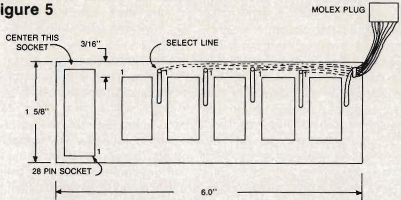
LEAVE RIBBON CABLE TO MOLEX PLUG 2 1/2" FROM BOARD. SLOT THE BOARD AND RUN RIBBON CABLE THRU AND UNDER THE BOARD. BRING EACH SELECT LINE THRU A HOLE ALONG SIDE OF THE SOCKET THEN BACK THRU THE BOARD TO PIN 20. THIS KEEPS THE WIRE DRESSED CLOSE TO THE BOARD. HOLD THE SIZE AND SPACING SHOWN TO PREVENT INTERFEANANCE WITH OTHER COMPONENTS AND TO ALLOW FOR FUTURE MODIFICATIONS.
