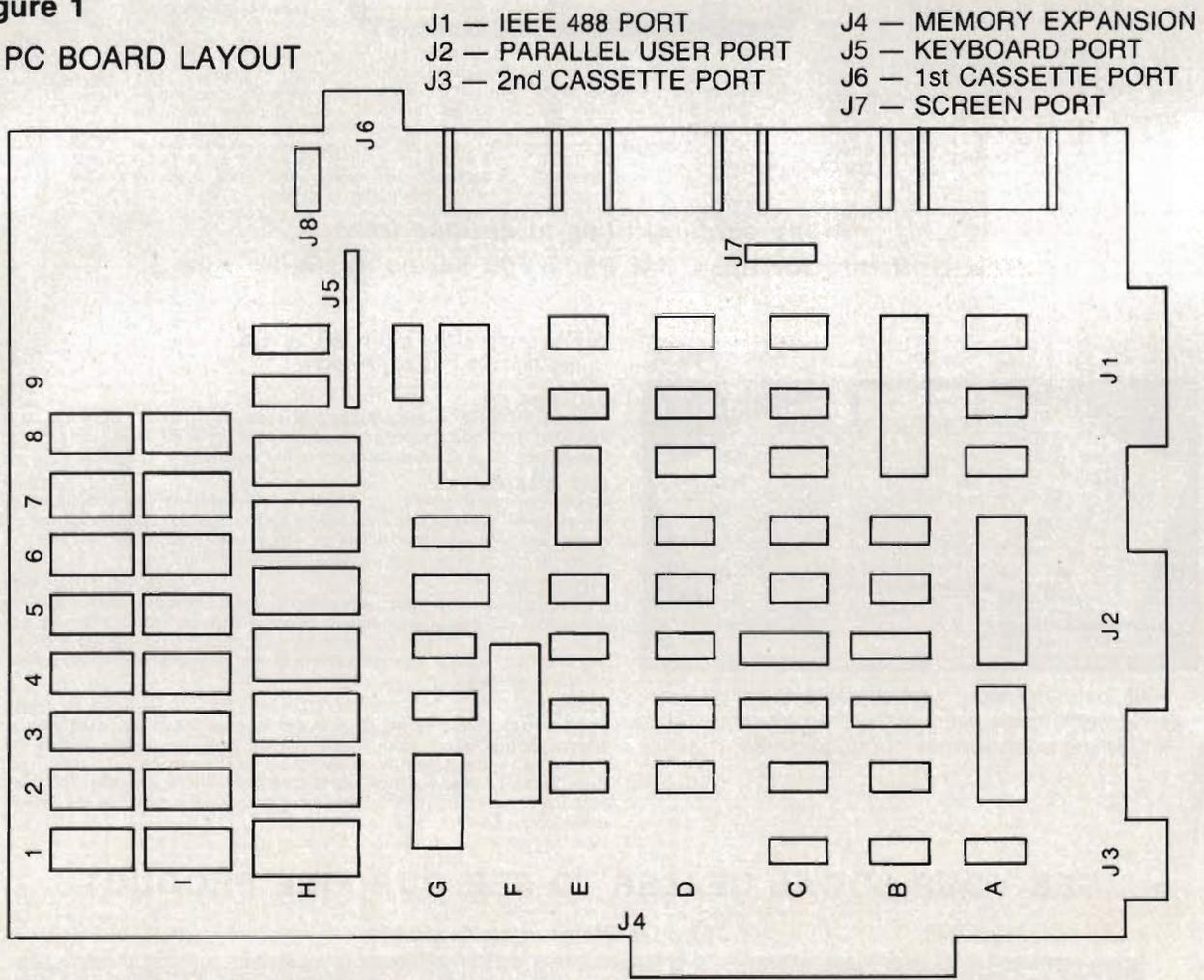
at G2. Located at G4 is a 74LS21 which is a 4 input AND gate that is used to select internal/external memory. The only internal memory blocks used by PET are 0, 1, 8, C, D, E and F. The balance is expected to be external memory to the computer selected
