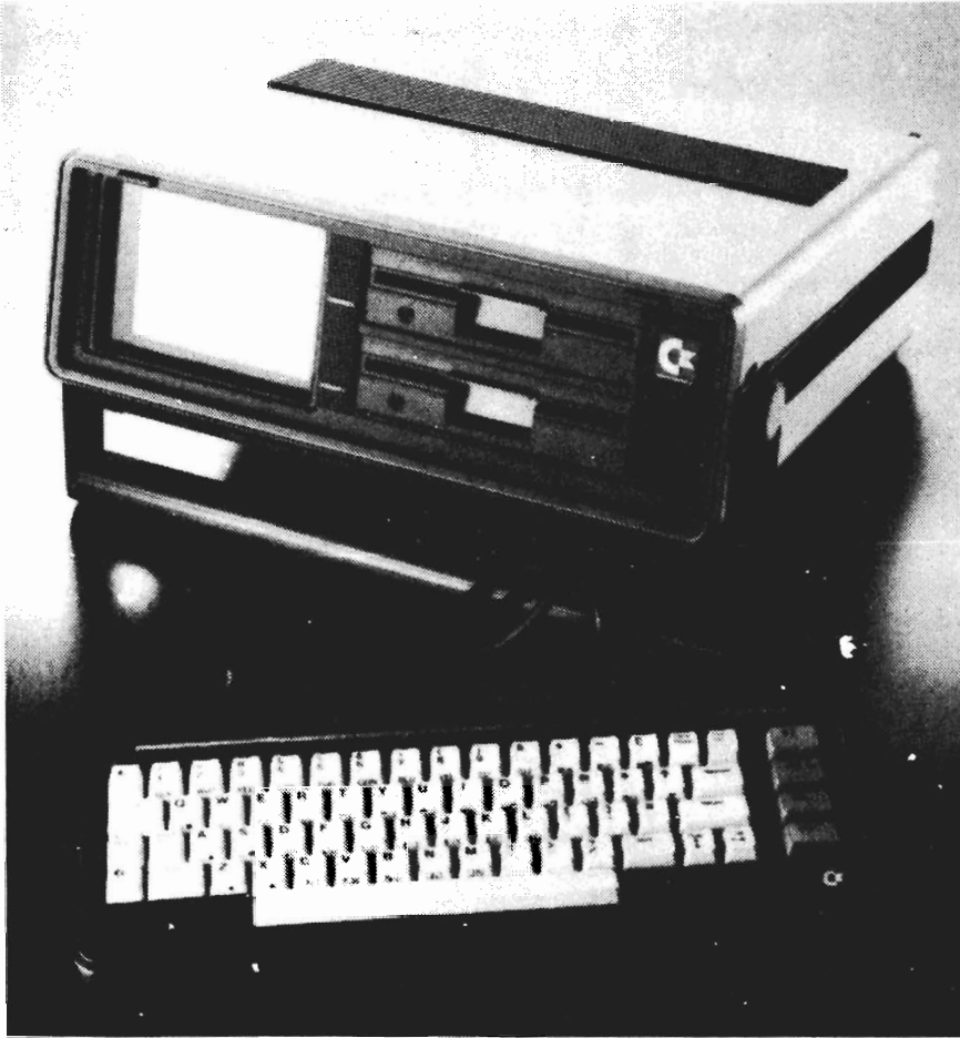
To the left: The Commodore portable Executive 64 weighing 27.6 pounds, travels easily. It has 64K RAM, a built in five inch monitor and floppy disk drives with 170K capacity.
