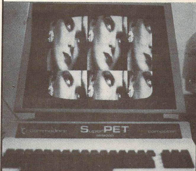
This is a graphics board which is universally compatible with all models of PET's. With Superpets (both 2 and 3 boards) It works equally well on both the 6502 and 6809 side as well as with OS-9.
