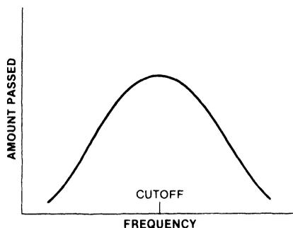
**Figure 11-11. Band-pass Filter**
