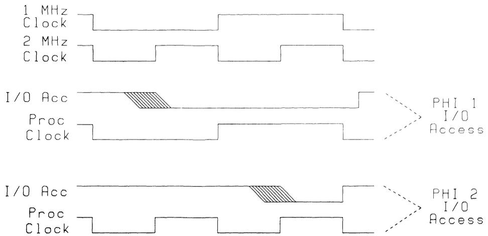
**Figure 16-4. Clock Stretching in 2 MHz Mode**
