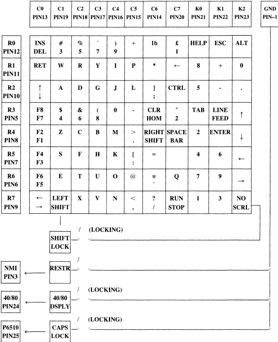
**NOTE:** Pins R0 through R7 pertain to the keyboard row values for the keyboard SCAN. These pins correspond to bits 0 through 7 of location 56321 (\$DC01).
