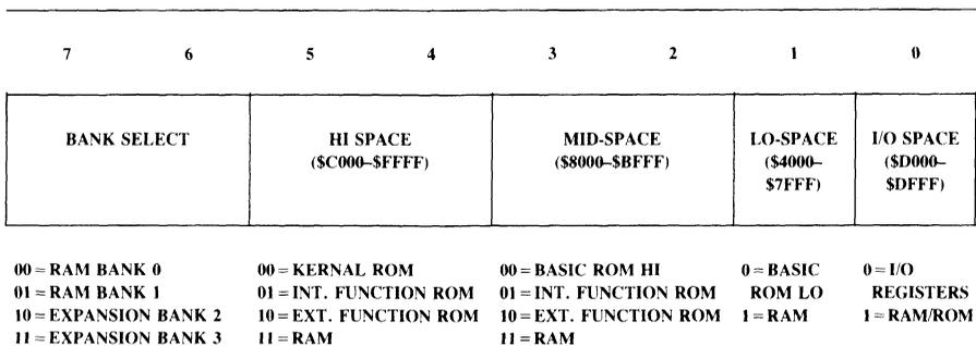
Figure 13-5. Configuration Register
