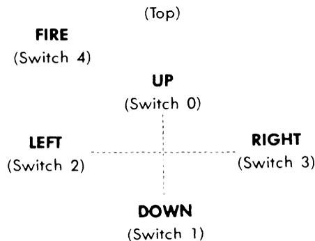
**Figure 12-4. Joystick Switch Arrangement**
