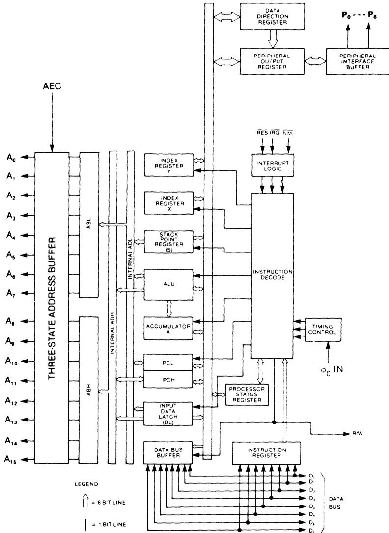
Figure 5-1. 8502 Block Diagram
