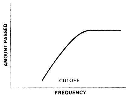
**Figure 11-10. High-pass Filter**
