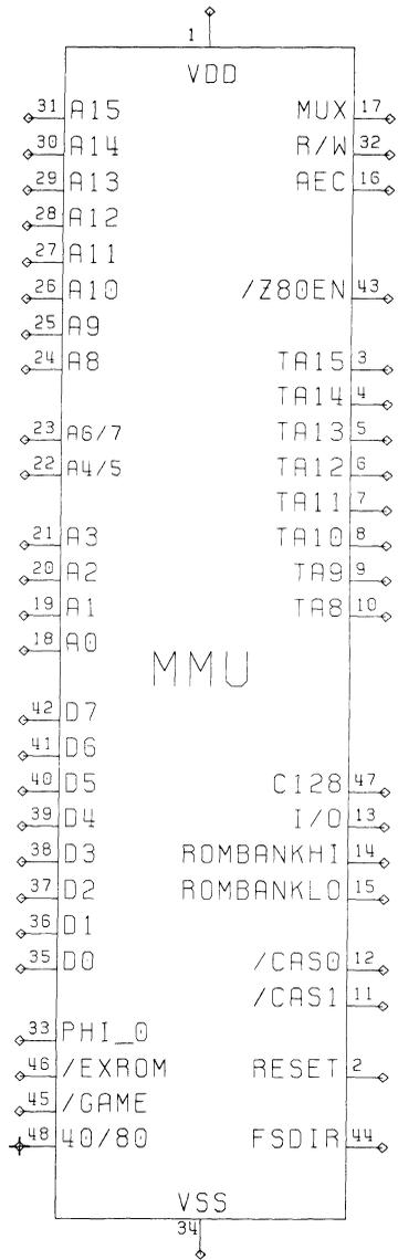
Figure 16-9. The Memory Management Unit Pin Configuration
