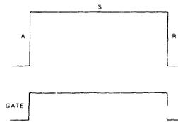
The real power of SID lies in the ability to create original sounds rather than simulations of acoustic instruments. The ADSR is capable of creating envelopes which do not correspond to any "real" instruments. A good example would be the "backwards" envelope. This envelope is characterized by a slow attack and rapid decay which sounds very much like an instrument that has been recorded on tape then played backwards. This envelope is shown below:
