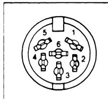
8. **Composite Video Connector**—This DIN connector supplies direct audio and composite video signals. These can be connected to the Commodore monitor or used with separate components. This is the 40-column output connector.
