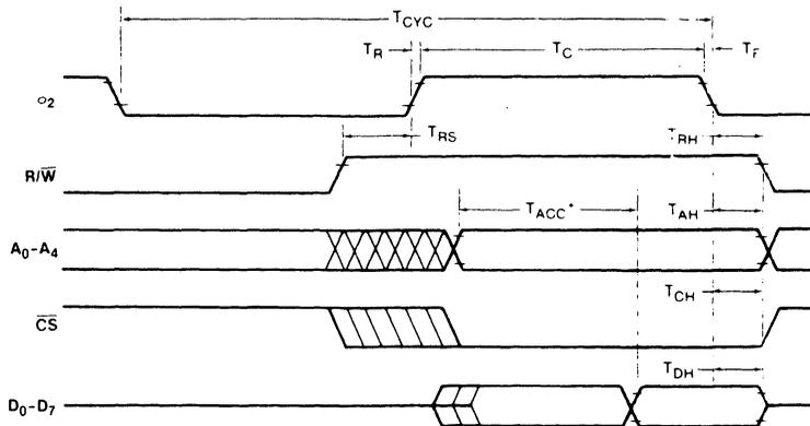
\* $T_{ACC}$  is measured from the latest occurring of  $o_2$ ,  $\overline{CS}$ ,  $A_0-A_4$ .
