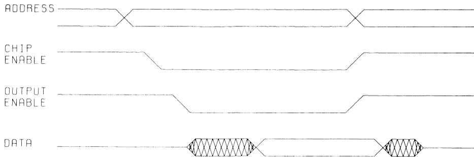
**Figure 16–25. ROM Timing Diagram**
