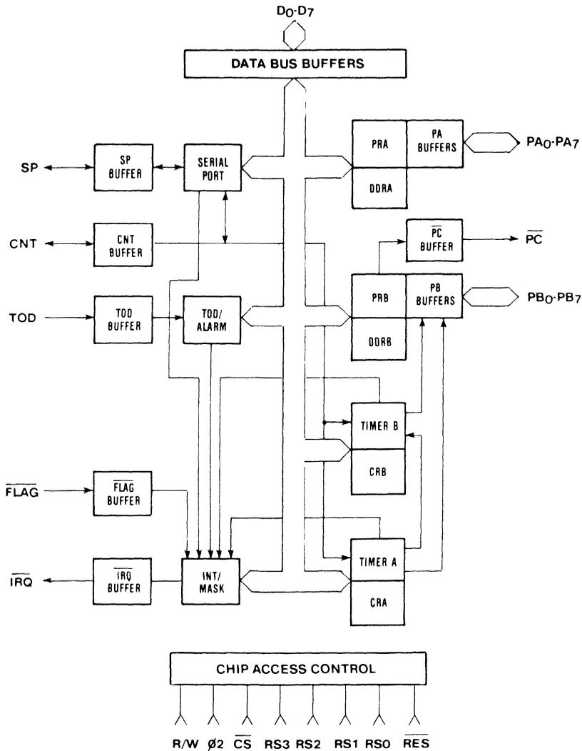
Figure 16-20. 6526 Block Diagram
