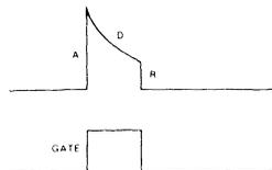
Note that the tone decays slowly until GATE is cleared, at which point the amplitude drops rapidly to zero.
