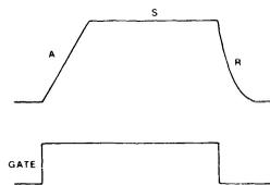
Many unique sounds can be created by applying the amplitude envelope of one instrument to the harmonic structure of another. This produces sounds similar to familiar acoustic instruments, yet notably different. In general, sound is quite subjective and experimentation with various envelope rates and harmonic contents will be necessary in order to achieve the desired sound.
