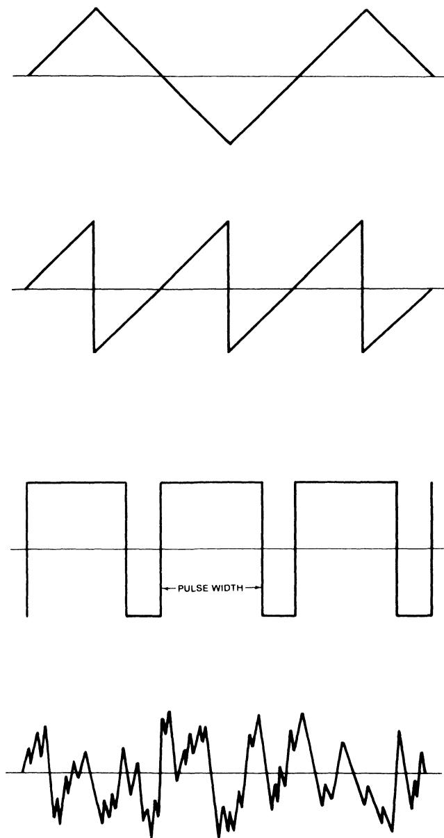
Figure 11-6. Sound Waveform Types
