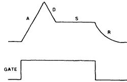
Note that the tone can be held at the intermediate SUSTAIN level for as long as desired. The tone will not begin to die away until GATE is cleared. With minor alterations, this basic envelope can be used for brass and woodwinds as well as strings.
