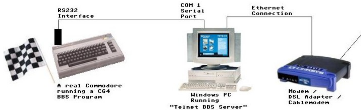
Figure 1 - Telnet BBS System Setup (Courtesy of www.telbbs.com )
