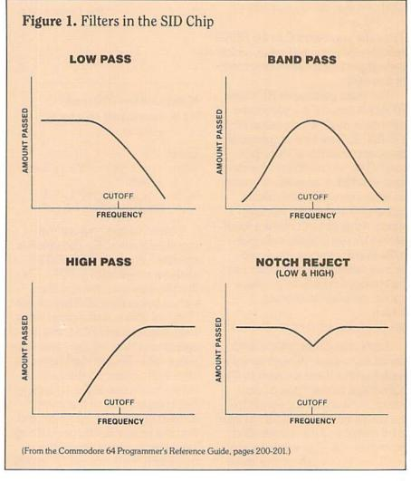
The addition of 16 to this POKE sets the filter to LOW PASS mode, thus quieting frequencies higher than the cutoff.
