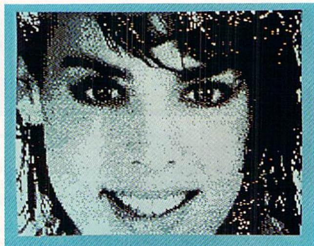
*Top left: Computereyes high contrast capture in Koala multicolor format. Top right: A 280 x 192 pixel image by Computereyes II and Spartan. Right: 8 level, 160 x 200 pixel Kinney image.*
