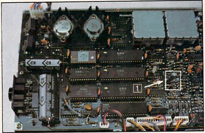
**PHOTO 4 (left):** Device number selection pads on long board; **PHOTO 5 (right):** ditto for short board.
