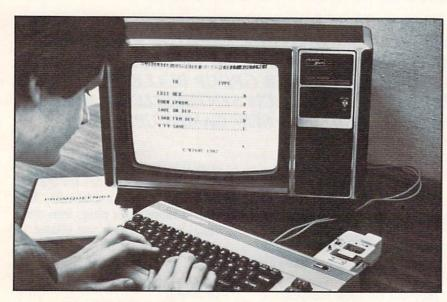
The Promqueen/64 is inserted into the expansion slot.
