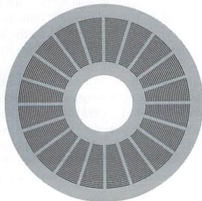
Data is written to disks in concentric rings called tracks. Each of the 'circles' on the disk diagram to the left is a track. Tracks are further broken down into more efficient storage areas called sectors. A single data block is read from or written to a specific track and sector location, also referred to as a track and sector address.
