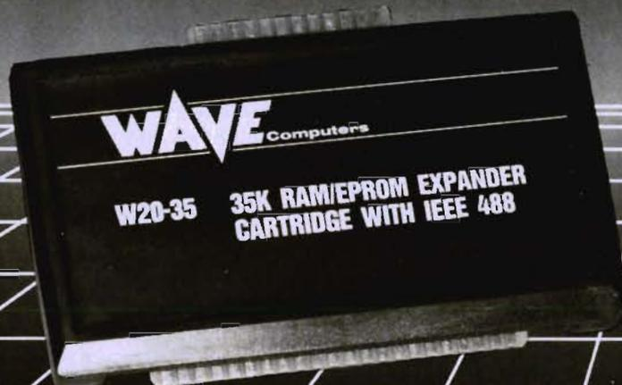
Your VIC 20 is expandable to 40K, but why buy four cartridges and an expansion chassis when you can have all this on one standard size cartridge; 35K of RAM or 32K of EPROM plus IEEE 488 interface for your hard disks, printers, and other peripherals.
