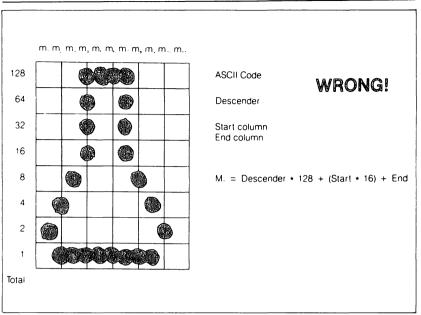
**Figure 5-6.** Dots cannot overlap; those in immediately adjacent "half columns" will be ignored when the character is printed.
