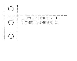
O | | LINE NUMBER 3, | LINE NUMBER 4. The form feed (CHR\$(12)) in line 60 caused the printer to move to the top of a new page before printing the last two lines.
