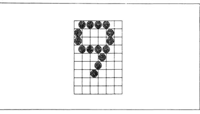
**Figure 5-3.** Dots can be inside boxes or straddle the vertical lines of the grid.
