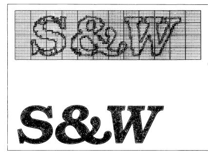
**Figure 6-2.** You have to sketch your design on graph paper before you can calculate the graphics data.
