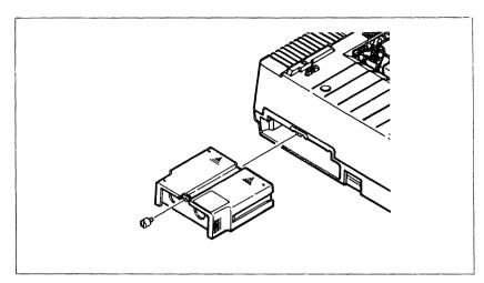
**Figure 1-1.** Slide the interface cartridge into the slot and fix it with a screw.
