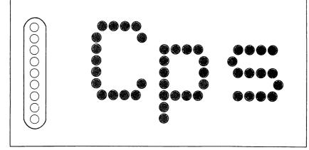
**Figure 5-2.** As the printhead moves across the page, each of the wires prints one row of dots.
