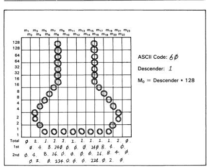
Figure 5-13. Add the values of the dots in each box and line column and write the sum of each column at the bottom.
