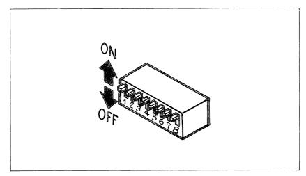
Figure A-1. The DIP switch is several small switches in one package.
