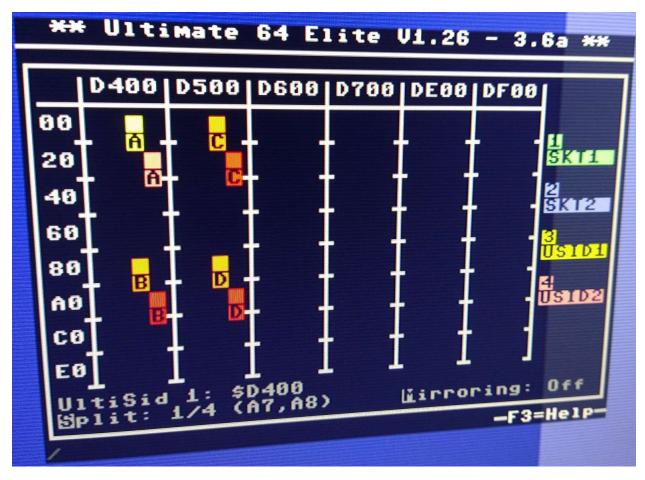
Since the split settings are shared for both UltiSIDs, UltiSID2 also gets split in the same way. But because its base address was set at \$D420 (A5=1), the splits appear also at offsets where A5=1, thus \$D420, \$D4A0, \$D520, \$D5A0. In total 8 SIDs, thus 24 voices and 8 independent filters.
