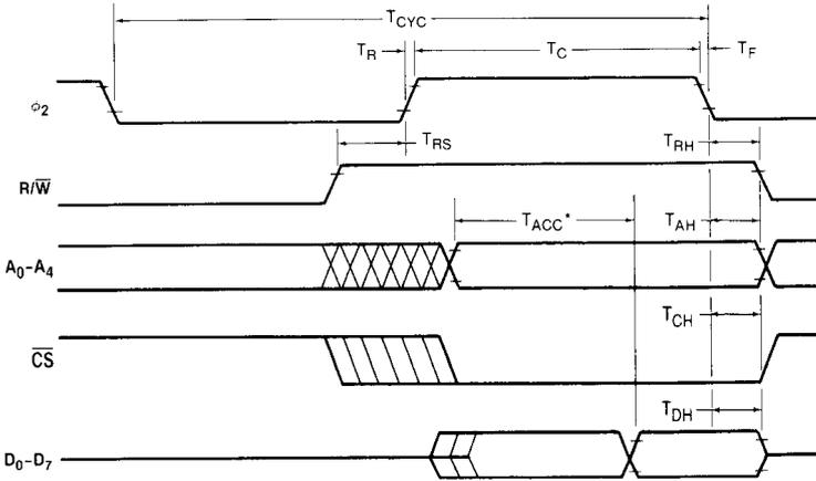
\* $T_{ACC}$  is measured from the latest occurring of  $\phi_2$ ,  $\overline{CS}$ ,  $A_0-A_4$ .
