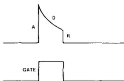
Note that the tone decays slowly until GATE is cleared, at which point the amplitude drops rapidly to zero.
