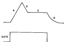
Note that the tone can be held at the intermediate SUSTAIN level for as long as desired. The tone will not begin to die away until GATE is cleared. With minor alterations, this basic envelope can be used for brass and woodwinds as well as strings.
