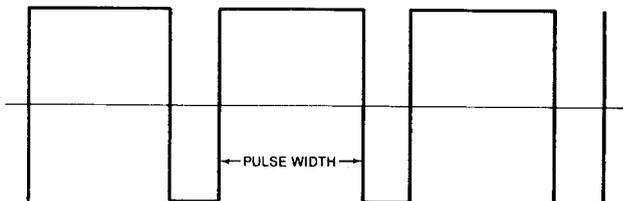
It is a rectangular wave and you determine the length of the pulse cycle by defining the proportion of the wave which will be high. This is accomplished for voice 1 by using registers 2 and 3: Register 2 is the low byte of the pulse width ( $L_{pw} = 0$  through 255). Register 3 is the high 4 bits ( $H_{pw} = 0$  through 15).
