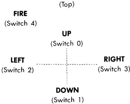
These switches correspond to the lower 5 bits of the data in location 56320 or 56321. Normally the bit is set to a one if a direction is NOT chosen or the fire button is NOT pressed. When the fire button is
