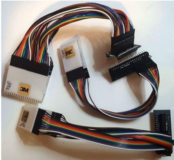
The **Clip Adapter** (one included with tester, additional clips available for purchase) provides a convenient way to attach a chip clip for in-circuit testing. You will need both a clip adapter and jumper extension wire for each chip clip you want to use.
