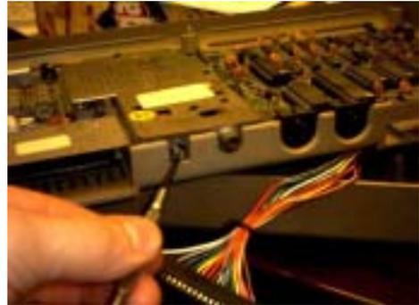
Now we can remove the keyboard from the top of the case this is held in by twelve Philips headed screws.
