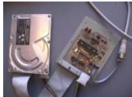
access an IDE hard device via the Commodore's normal disk drive serial port. Go to <http://www.djupdal.org/cbm/iecata/> to read about it. **CS** will cover this in a future issue.
