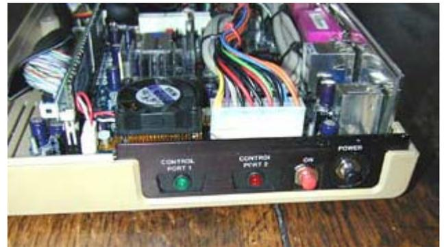
Cables were soldered on the leds and switches and plugged in the board. The original power led on top of the C64 casing was connected to the harddisk led output. That way the disk activity can be easily monitored.
