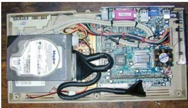
On the right side the original C64 metal lid can be seen. Normally this would house the power connector, power button and the two joystick ports. I converted it by glueing a piece of aluminum on the
