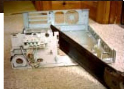
I decided to hold the motherboard in place with self-tapping screws. The screws were positioned from the top in to the plastic of the p.c. case. I had to cut away some of the case rear for the joystick connectors to fit through and the power. I slightly cheated here as I am still using the Commodore power supply and didn't even try using the
