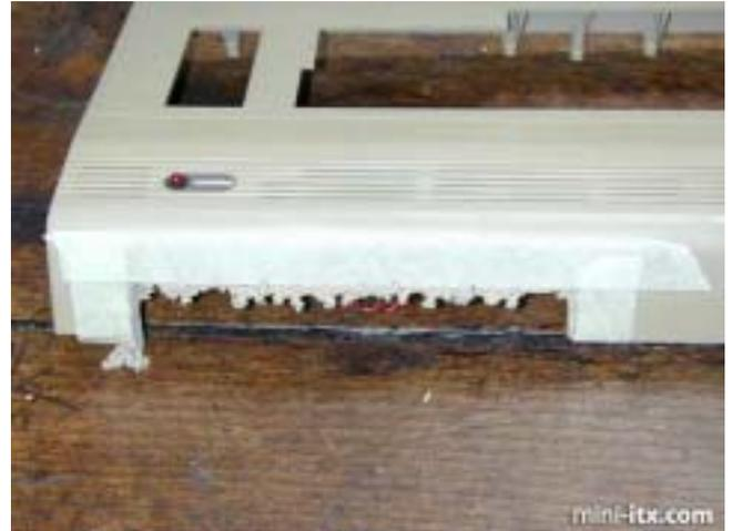
The end result after one hour of filing the plastic with delicate instruments can be seen below. Yes, this is going to be good. You will notice that the two lids articulate at an angle (approx. 10 degrees) while the backplate is straight. I do not recommend you trying to bend this plate as it is rather fragile and will probably break. It fits OK though, as you can see:
