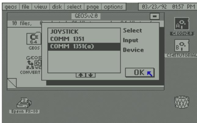
A new box will appear with a list of input drivers in it. Select the **COMM 1351(a)** driver and click on the **[OK]** box. The mouse driver will be installed and the icon will be moved to the front of the disk.
