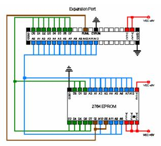
Now that we have designed the cartridge and hopefully programmed the EPROM correctly all that is left for us to do is solder the EPROM to the PCB. That's it. You now have a working 8 K cartridge for the Commodore 64.
