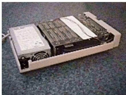
Figure 2 - It is a very tight installation but with the correct PCB you can fit the FDD, HDD and PSU.
