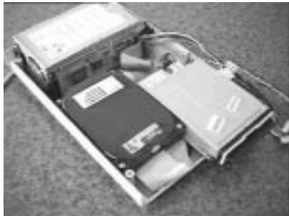
install the plug. I found mounting the drives in a staggered and opposite facing way gave me the easiest result. This also allows the FDD to protrude through the 1571 fascia, whilst the HDD is hidden inside.
