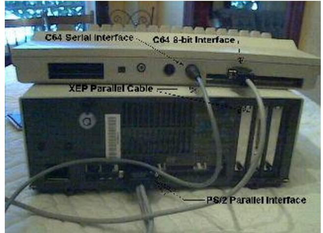
The first and easiest option is to buy yourself a cable and simply plug it into the LPT card and drive. There are various re-sellers for this cable and so finding one shouldn't be a problem. This method though has one small drawback, the standard cable provides only one serial connection.
