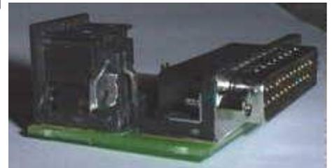
The third method requires some soldering skills and involves connecting the individual wires from the cable directly to the LPT connector inside the PC's case. This gives the neatest result and is the method I have used on the 64HDD system housed in a 1571 case. You can have connections to multiple sockets if needed.
