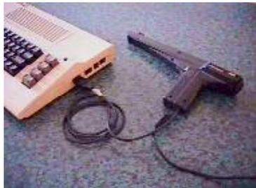
instructions include pinout information for the adaptor and a BASIC demo/test program for the LightPen mode. Note that only Control Port#1 on the C64 is connected to the Light Pen input on the VIC chip. Standard Light Pen software will also work with the Light Phaser.
