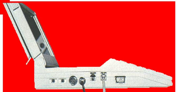
Unlike the SX64 the Commodore LCD is battery powered. There's a device for four 1,5V batteries which guarantees real portability. Yes, you are right: there is no harddisk inside the LCD, so where do we store the things we already worked at? (Assuming we were proud owner of this pretty machine ;-)
