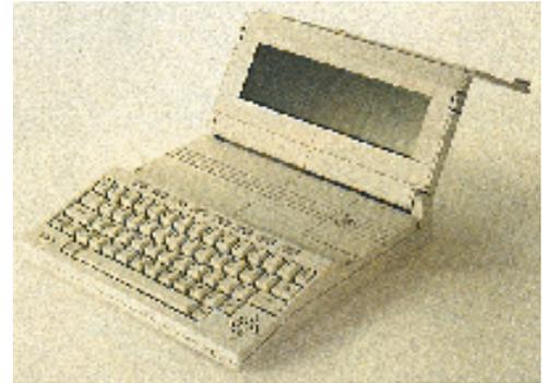
The Commodore LCD has a monochrome 'Liquid Crystal Display' (short 'LCD') which is able to show 80 characters x 16 lines in text mode or 480 x 128 pixels in graphics mode. Thus, one character consists of 6 x 8 pixels which results in a very narrow character set (at least in comparison to the C=64 which has an 8 x 8 pixel character matrix). Nevertheless you can recognize the characters very well.
