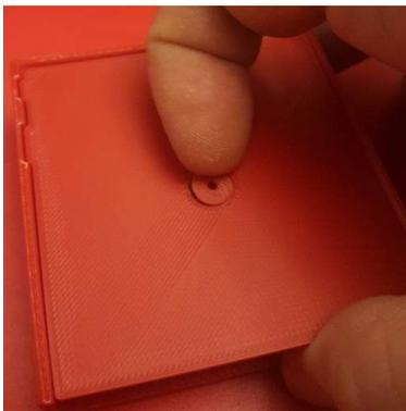
1. Use fingernail to remove peg from the back of the cartridge. Don't lose it!
