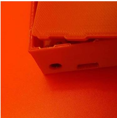
6. Line up the back plate, aligning the 2 small notches as shown. Screw the plate in by hand, being careful not to over-tighten (the program button can get stuck if it is).
