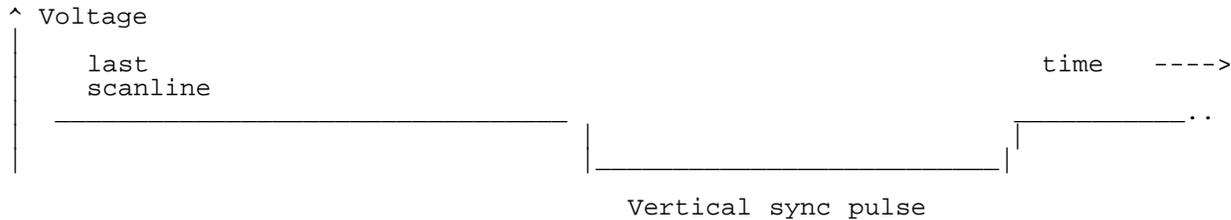
We end up with a vertical sync pulse that looks very much like the horizontal sync pulses, except it runs at a much lower frequency. In NTSC, the field frequency is 60 Hz, and the frame frequency is 30hz (PAL has a 50Hz field rate and 25Hz frame rate). In other words, we get one of these vertical pulses on every field, to let the TV know when the field starts (just like the horizontal sync pulses tell it when a line starts). According
