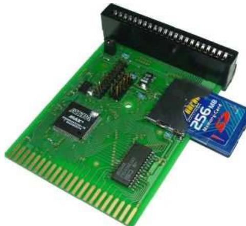
The latest expansion (only!) for the MMC64 is called MP3@64. It is an MP3 expansion module for the clock port connector featuring a DSP and a 20-bit D/A converter, enabling the Commodore 64 to play MP3 files in CD quality!
