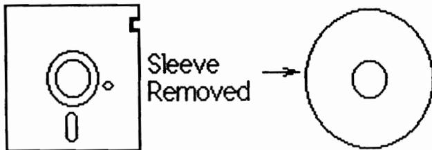
The 1541 divides a disk into 35 concentric circles, called tracks. The inner tracks are smaller in circumference than the outer ones. The 1571 does the same to both sides of a disk, and the 1581 has 80 tracks.
