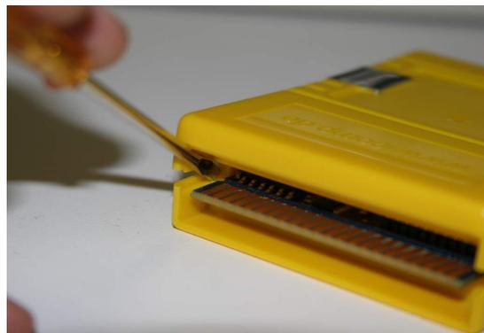
With the opening in the Chameleon case for the mini-DIN connector, the left half of the case top is fairly weak. We therefore recommend to open the right side of the case first:
