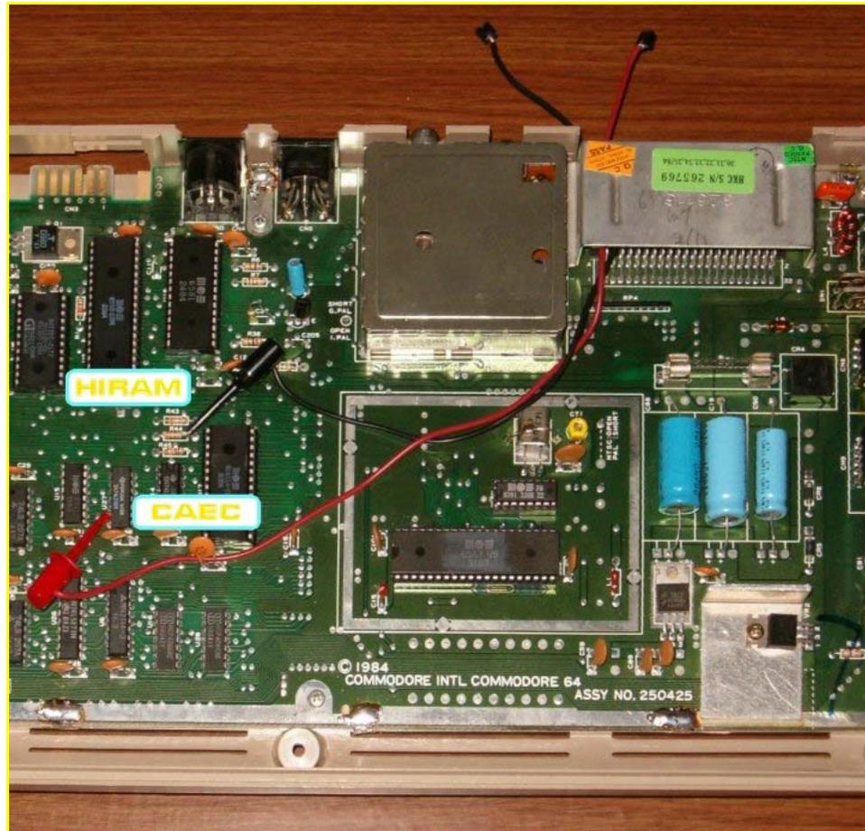
The Mini-Clip Connections for a C64 (or 64C) can be done in Just Minutes.
