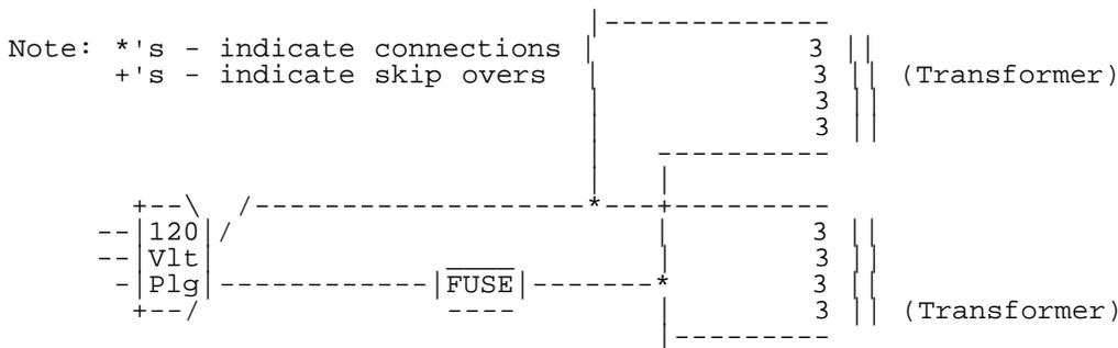
This would now be a good time to install a fuse in your 120 VAC line. Now before plugging this into the wall, tie two of the scndary leads (one from EACH transformer) together.
