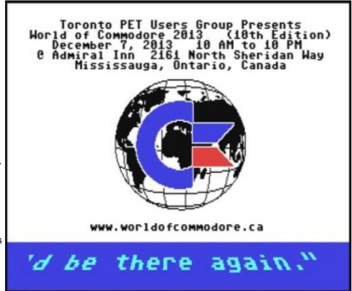
The scroller uses 16 lines of graphics and each line gets a different (virtual) pixel width. This makes the bottom line look like it's scrolling faster. The graphics in the bottom line also looks wider.
