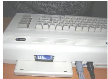
Figure 4 - Cutout above cartridge slot for Compact Flash card
