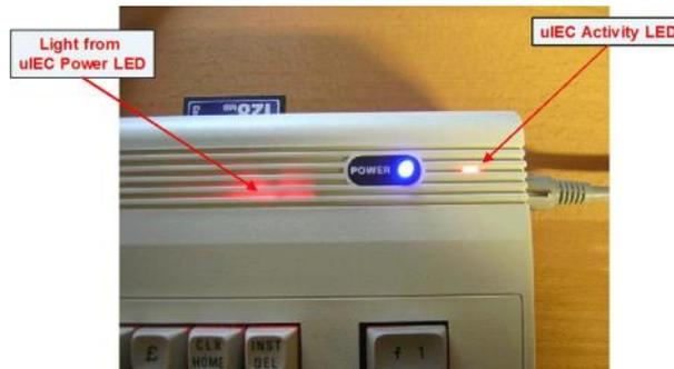
Figure 2 - Blue Power LED and activity LED from uIEC
