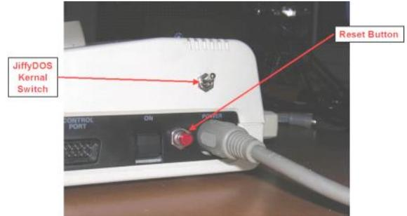
Figure 3 - JiffyDOS switch and reset button
