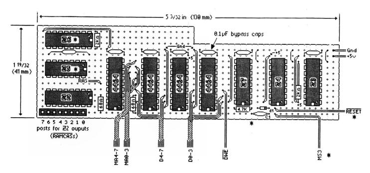
\* ICs Z5, Z6, Z7, associated components and signals required for 512K only. Note reversed locations of +5v and ground for DRAMs.
