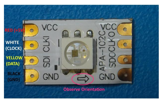
For an easy connection of the LED strip, it is recommended to connect four wires / leads to it, with a single pin socket, like the ones shown below. These wires can be obtained anywhere, and are sold -for example- as Raspberry PI jumper cables.
