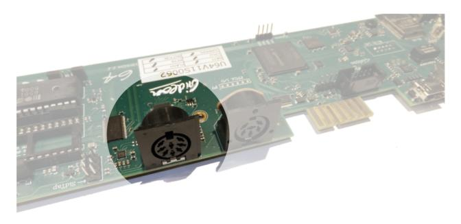
The 8-pin DIN ( audio/video ) connector can output several different video signals, for each type you need a special assembled cable.
