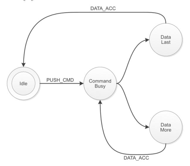
Figure 1: Basic Protocol State Machine
