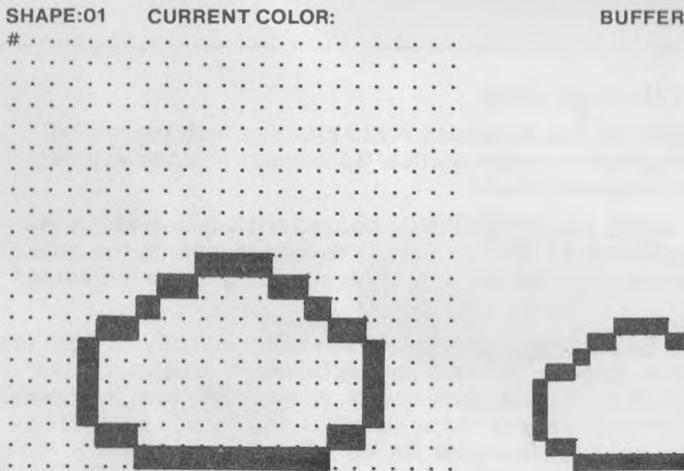
A number sign (#) indicates the current cursor position. The filled in spaces indicate the pixels that are turned on, thus giving the sprite its shape. The + key cycles forward through the sprite shapes, and the - key cycles back.
