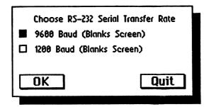
Select either 9600 or 1200 from the dialog box. 9600 is the normal setting for use with geoPubLaser, since it is eight times faster than the 1200 baud rate.
